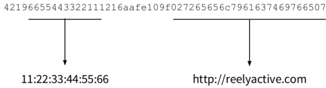
Fig. 3. Raw BLE packet split into 48-bit identifier and Eddystone URL
